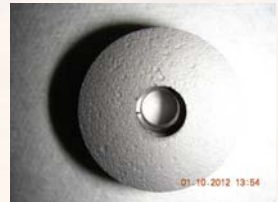
Figure 1: Sample Part Drawing/Photo of Sample with Helicoil Insert
